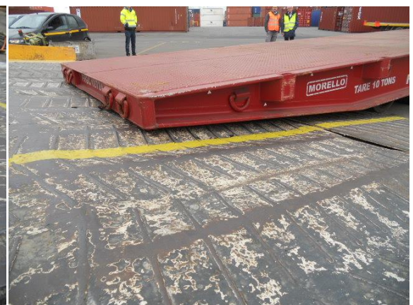
Fig.4 – Operation of loading / unloading INCORRECT
